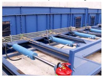
The Moving floor system is equipped with a hydraulic power unit for generating the oil flow to the hydraulic cylinders.
